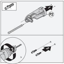
into wall. Install anchors.
