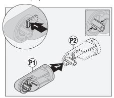
**Note:** Mounting plate (P2) center tabs must be horizontal for removal.
