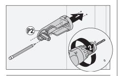
**Option:** Place mounting plate (P2) in position, mark and drill 3/16" holes
