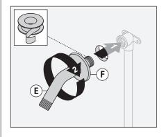
13) Install showerhead (D) to shower arm (E) turning clockwise to tighten.
