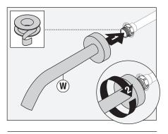
Install wall elbow (B) and flange (C) to recessed pipe fitting. Turn elbow clockwise to tighten.
