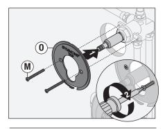
3) Attach diverter escutcheon (N) to plastic mounting plate (O).
