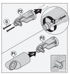
Replace cradle mount cover (P1). **Note:** Mounting plate (P2) center tabs must be horizontal for installation.
