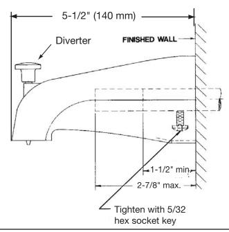
**Caution:** Ensure seal is not damaged by making outside of 5/8 inch diameter tube is free of burrs and sharp edges prior to tub spout installation. Tube length from finished wall should be 1-1/2" min. to 2-7/8" max.
