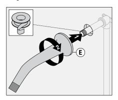
9) Install showerhead (D) to shower arm (E). Turn clockwise to tighten.
