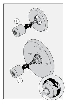
5) Install diverter handle (5205 and 5206 only) (G) and shower handle (M) to valves. Secure handles by tightening set screws (H) and (N).
