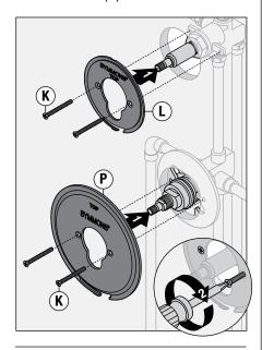
2) Attach diverter escutcheon (J) to small plastic mounting plate (L).
