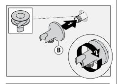
8) Attach shower arm (E) to vertical shower pipe. Turn clockwise to tighten.
