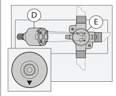
**Note:** For diverter valves purchased before November 2016, retaining sleeve (F) must be inserted flush into diverter valve (E) before installing cartridge (D).
