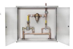
and fittings to cabinet limits. Standard rough bronze and copper finish. Bottom supplies and top outlet. Factory assembled and tested. Cabinet to be 16 gauge (1.6mm) body, 12 gauge (2.7mm) left hinged door (or double doors on larger systems) with cylinder lock and key. Standard cabinet fully recessed steel, with baked white enamel finish.
