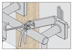
9) Apply a bead of silicone around the perimeter of the Toilet Paper Holder ends to prevent water from bleeding through the mounting holes and potentially damaging the wall and wall studs.
