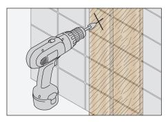
Follow step 1 for wall and wall studs to mark centers of Toilet Paper Holder ends. Use drill with 5/16" carbide tip drill bit to drill holes into ceramic tile at the marked positions to prevent damage to the tiles.
