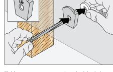
5) Keep pressure on bar behind the drywall. Align holes in bar, white flange and bracket. Align machine screw with holes. Hand tighten machine screw so bar remains upright.
