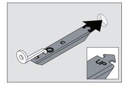
3) Hold white flange upright and insert mounting anchor bar into drywall hole with the arrow facing toward the drywall.
