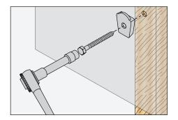
Use ratchet and lag bolt to attach mounting bracket to wall. Do not overtighten. Repeat step for opposite end, and then tighten both brackets so they are secured to wall.
