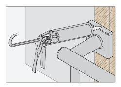
6) Apply a bead of silicone around the perimeter of the Toilet Paper Holder ends to prevent water from bleeding through the mounting holes and potentially damaging the wall and wall studs.
