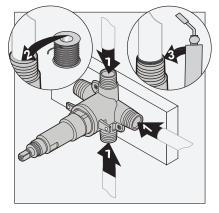
Turn on water supplies to flush plumbing lines free of debris. Check for leaks.
