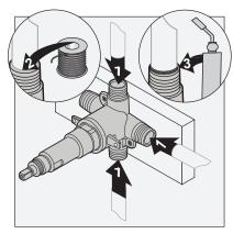
6) Turn on water supplies to flush plumbing lines free of debris. Check for leaks.
