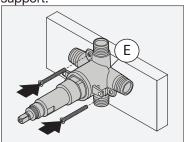
Note: Securing stringer mounts is necessary for applications where PEX, or other non rigid tubing, is used to install diverter valve.
