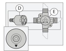
Important: Cartridge (D) must be installed with arrow facing down.  Align spindle extender (C) with broach on cartridge (D). Install spindle extender (C) and cap assembly (A) to cartridge (D). Secure cap assembly (A) by turning clockwise.
