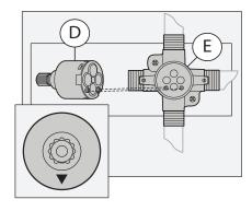
Important: Cartridge (D) must be installed with arrow facing down.
