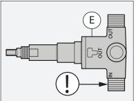
**Optional:** Apply plumber tape to male IPS threads on the inlet and outlet ports of diverter valve. Install 1/2"-14 NPT copper fittings to the inlet and outlet ports. Connect outlets to desired accessories.
