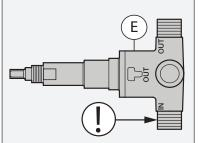
**Optional:** Apply plumber tape to male IPS threads on the inlet and outlet ports of diverter valve. Install 1/2"-14 NPT copper fittings to the inlet and outlet ports. Connect outlets to desired accessories.
