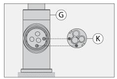
replace cartridge if necessary. Align pegs on cartridge (K) with holes in faucet body (G) as shown above.
