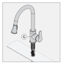
2) Install faucet body (G), supply hoses and pull-down hose to deck surface.
