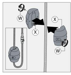
5) Attach counterweight (X) to outlet end of pull-down hose. Counterweight should be placed above the hose loop. Secure with 2x screws (W).
