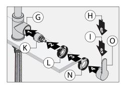
3) Replace cartridge (K), compression nut (L), collar (N), handle (O), set screw (I) and plug button (H).
