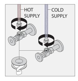
6) Connect hot supply hose (red stripe) and cold supply hose (blue stripe) to supply outlets.
