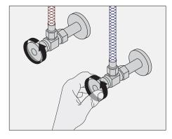
8) Turn on water supplies to flush lines.
