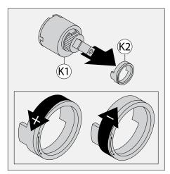
1) Remove limit stop (K2) from cartridge (K1). Turn limit stop counterclockwise to allow full handle turn to the hot position. Turn limit stop clockwise to limit handle turn to the hot position.
