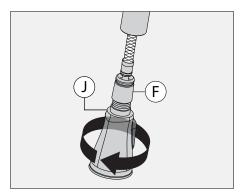
7) Remove spray wand (J) from pull-down hose coupling (F).
