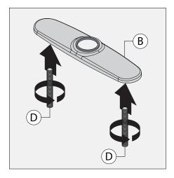
1) Thread studs (D) into deck plate
