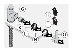
1) Remove plug button (H), set screw (I), 2) Inspect cartridge (K) for debris and handle (O), collar (N), compression nut (L) and cartridge (K) from faucet body (G).
