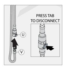
4) Attach outlet end of pull-down hose (V) to hose adapter (U). Press tab on hose adapter (U) to disconnect as shown above.
