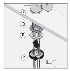
3) Install rubber washer (Q), metal washer (R) and mounting nut (S) to faucet body (G). Secure to bottom of deck with 3x mounting screws (T).
