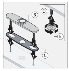
2) Install deck plate (B) and gasket (C) to deck surface. Thread mounting nuts (E) to studs (D) to secure deck plate (B) under deck.
