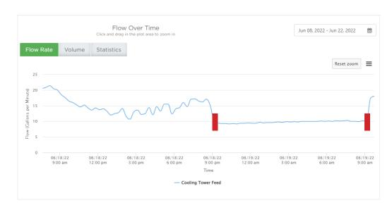
Using this data from the Evolution Dashboard, the property management's engineer quickly discovered that a mechanical control valve that regulated the water consumption for the cooling tower was broken. Witnesses on scene reported that after repairing the part that day, water usage dropped to zero that night:
