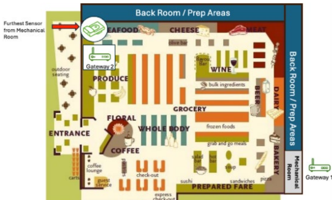
Figure 8. Suggested gateway locations in a typical store layout.
